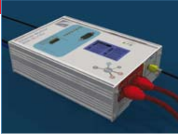
Ethernet Monitor for timing analysis and tracing of Industrial Ethernet protocols
